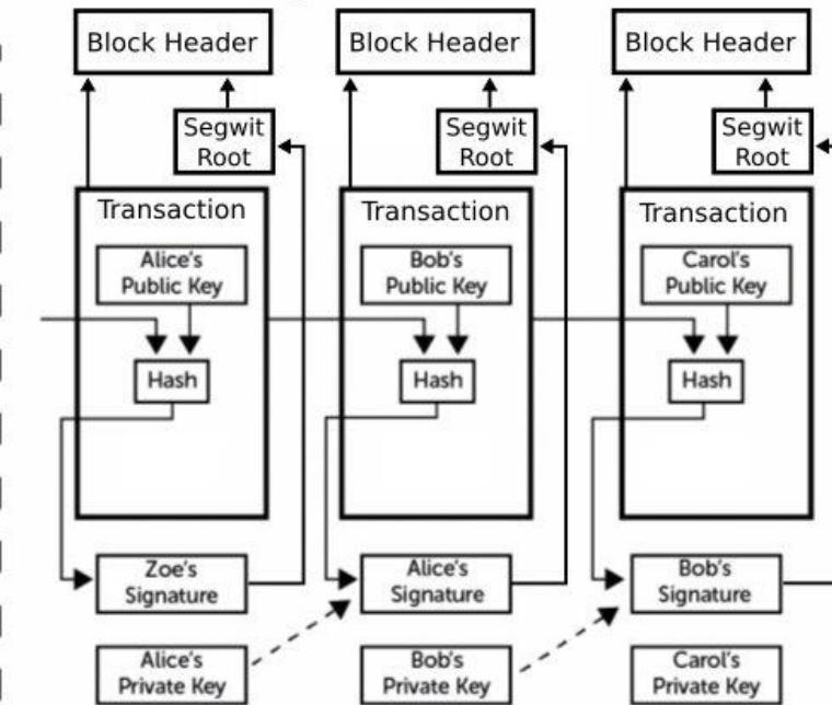
Each block header still includes a cryptographically-secured reference to all of the transaction data in that block, but encumbrances (public keys) are referenced separately from witnesses (signatures) so that software can use each part independently.
