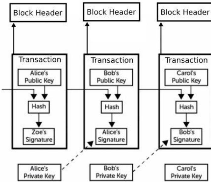
Each block header includes a cryptographically-secured reference to all of the transaction data in that block.
